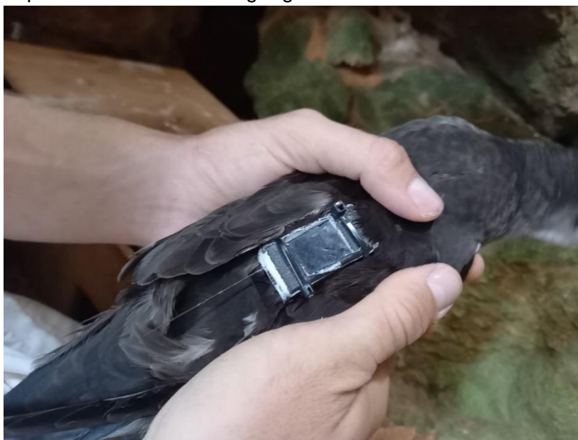
Figure 1: The GPS device, Axy-Trek (TechoSmart Inc, Rome, Italy) with a solar panel, attached to the back feathers of a Yelkouan Shearwater using Tesa® tape (Tesa SE, Hamburg, Germany). The picture shows an individual breeding within the largest colony of Yelkouan Shearwaters in Malta, situated Rđum Tal-Madonna. It was tracked as part of the project LIFE PanPuffinus! (LIFE19 NAT/MT/000982)
