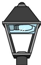
fully shielded 'period' style fixtures
