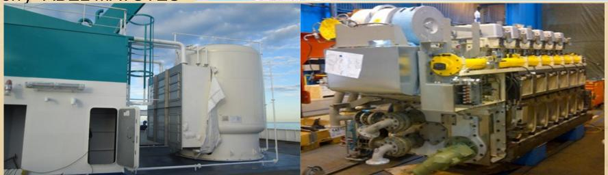
LNG Port Aux. generator: Rolls-Royce Bergen C26:33L6AG: 1.620 KW
