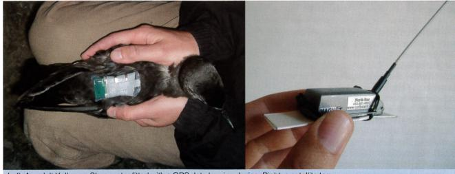
Left: An adult Yelkouan Shearwater fitted with a GPS data logging device. Right: a satellite tag
