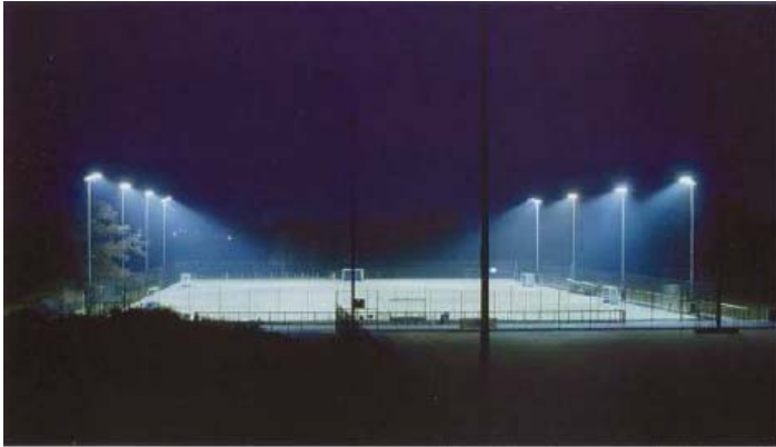
Figure 1: Example of good lighting shining downwards. Source: Abacus Lighting.
