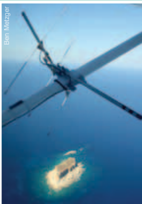
▲ A Cessna wing strut with Yagi-antenna during a radio-tracking flight over Filfla.
